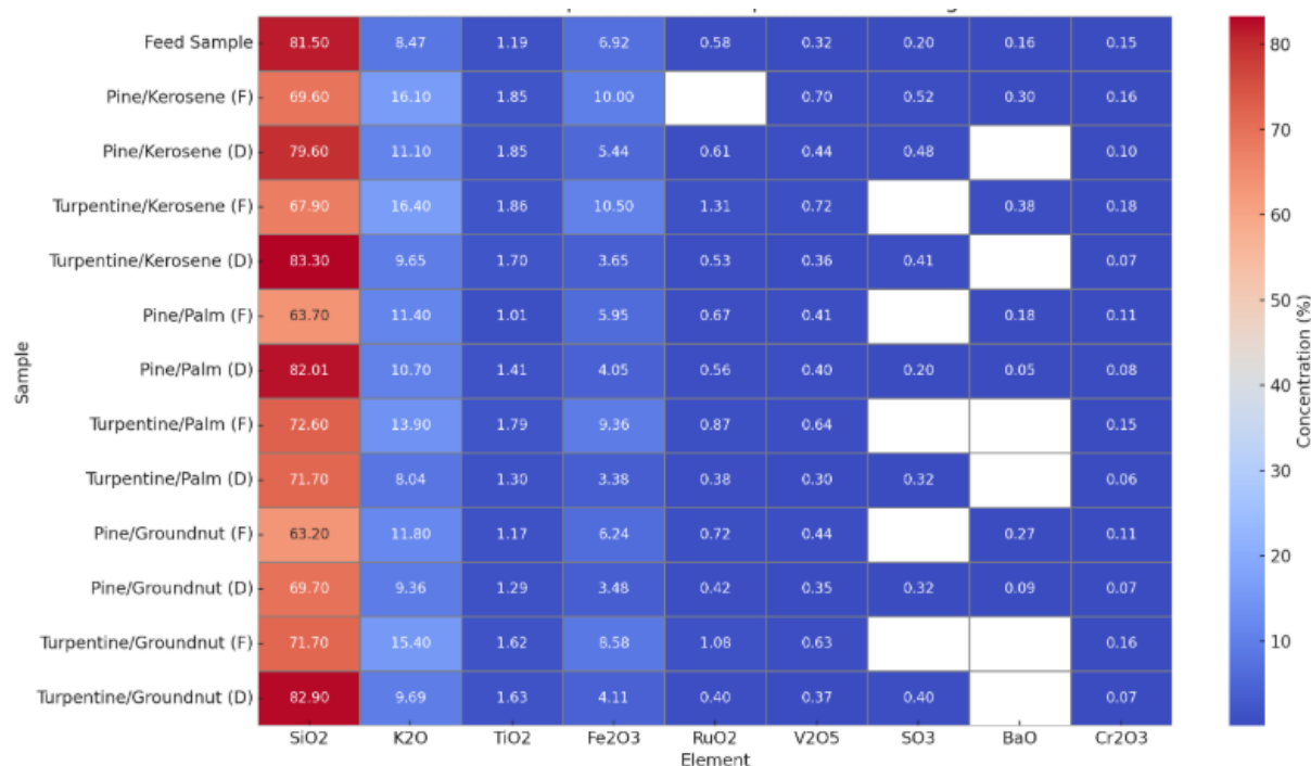
Figure 3. The heat map delineates the elemental composition of the Ningi graphite feed sample, establishing a correlation with both the froth (F) and depressed (D) products derived from conventional and environmentally sustainable graphite flotation systems.
