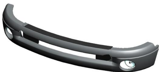
Figure 2. 3D modelling, Isometric view of frontal bumper cover model.
