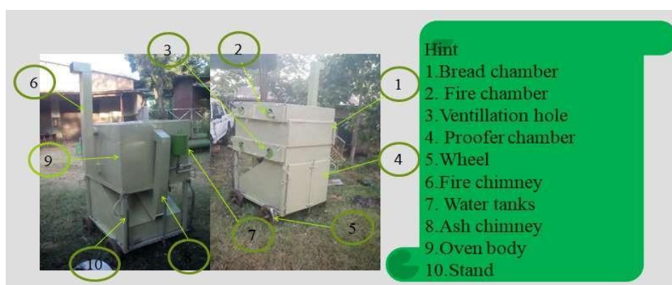
Figure 1. View of the Portable Wood Powered Bread Baking Oven Components.
