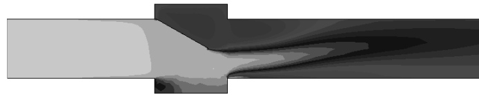
Figure 9. Total pressure field at the intermediate time t = 0.11s(\theta = 330^\circ) .
