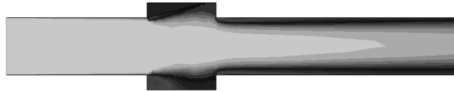
Figure 10. the total pressure fields at the fully open time t = 0.18s(\theta = 370^\circ) .
