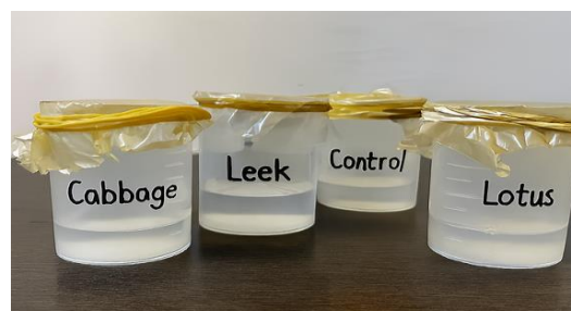
Figure 3. Estimation of the Water Vapor Transmission Rate of the Prepared Coatings.
