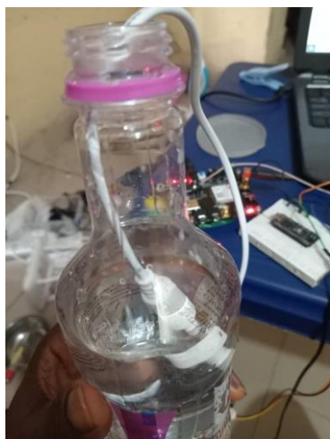
Figure 8. Image of the TDS/EC sensor is used to measure the TDS or electrical conductivity, EC value of water.
