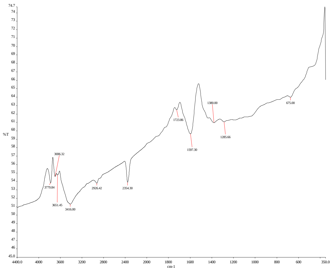
Figure 13. FTIR spectrum of the residue gotten from Cu NPs ( Mimusops coriacea )/Mixed dye.
