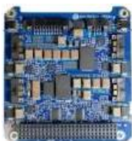
Figure 8. GAUSS PCDU PDB Board.
