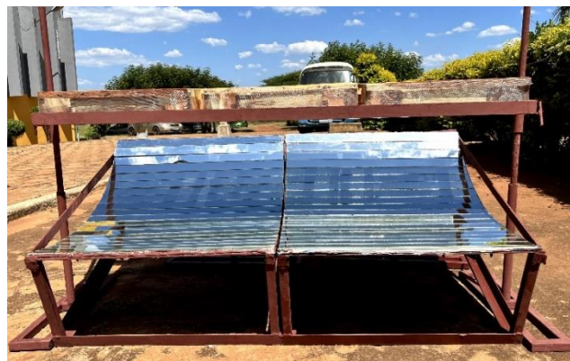
Figure 9. Dryer connected to the solar concentrator in operation.
