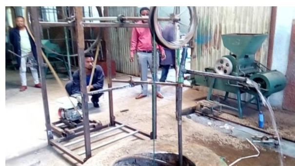
Figure 4. The modified engine driven rope and washer pump.
