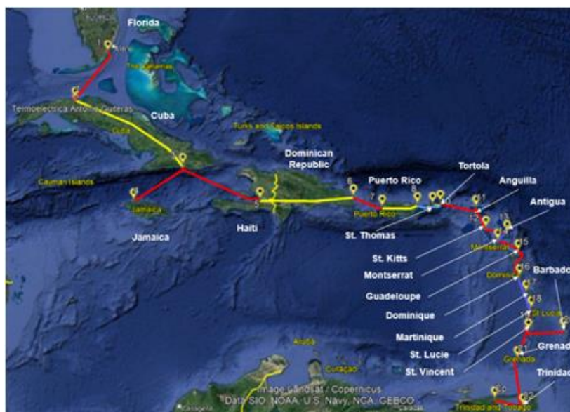
Figure 1. Schematic representation of the interconnection of the Caribbean electricity markets.
