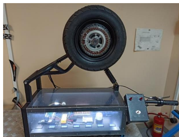
Figure 3. Photograph of a test stand for an experimental model of a motor-wheel made of a soft magnetic composite material.
