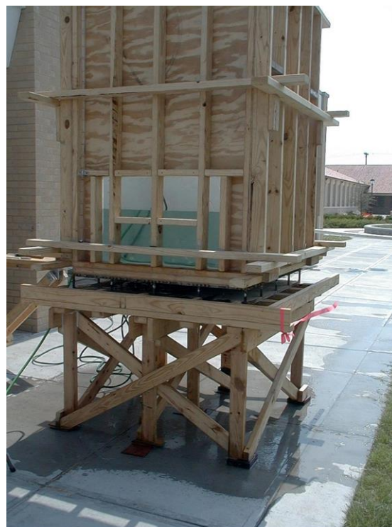
Figure 5. Experimental setup showing water tank on the scaled flat plate slab.
