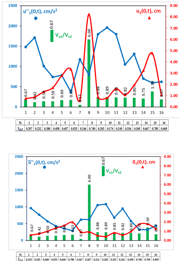
Figure 7. a. Peak values of accelerations u''_1(0,t) (cm/s 2 ) and displacements u_1(0,t) (cm) for the 16 variants (Figure 3.) of actual two-layer heterogeneous foundation beddings, and, b. equivalent single-layer homogeneous foundation beddings, depending on the ratio v_{s1}/v_{s2} , T_{01} , \bar{T}_{01} and No. of foundation (considering three oscillation modes at M=7.0 , A=15 km, \Theta_1=\Theta_2=\Theta_3=0.3 ).
