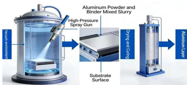
Figure 4. Schematic Diagram of Vacuum Spray Coating Principle.
