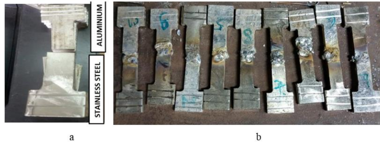
Figure 7. Specimen: a-Different metals and b-Welded dissimilar metals.
