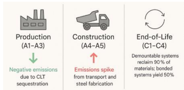
Figure 3. Life Cycle Stages of Steel-CLT Systems. (Adapted from [6]).
