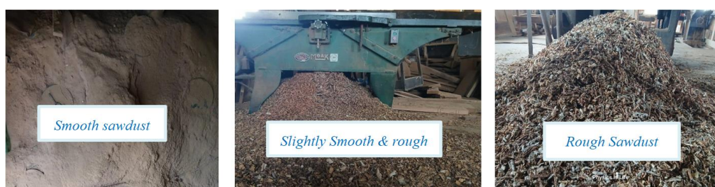
Figure 6. Sawdust with different Densities and Sizes from the ETU-SL Carpentry Workshop.
