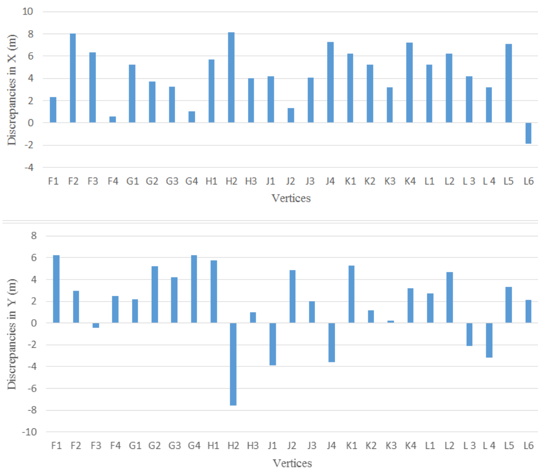
Figure 3. Relative discrepancies in coordinates acquired through direct survey in RTK NTRIP mode and those derived from Google Earth along the X and Y axes in Abomey-Calavi.
