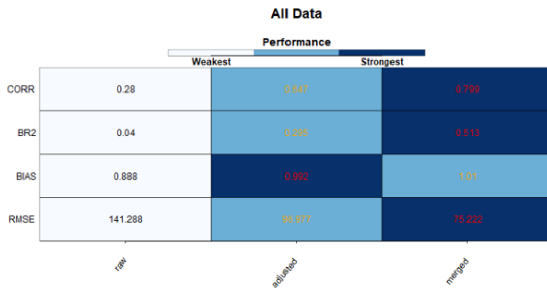
Figure 4. Performance rank of raw, adjusted and merged datasets in reproducing the observed precipitation data.
