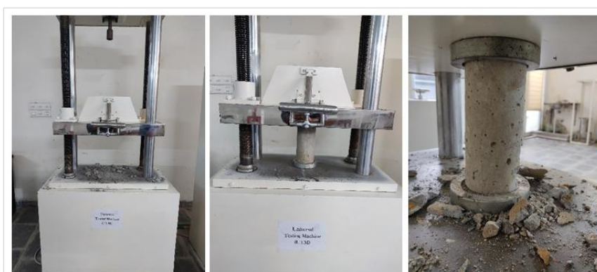
Figure 4. Compressive strength checking by UTM machine.
