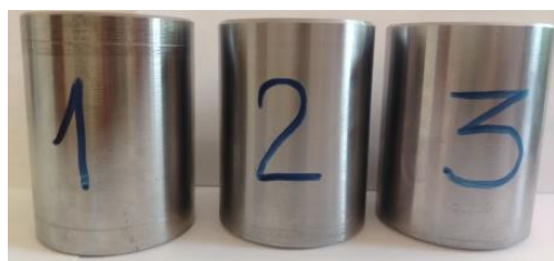
Figure 3. Outer bushing of the working body support structure for a vertical shaft machine.
