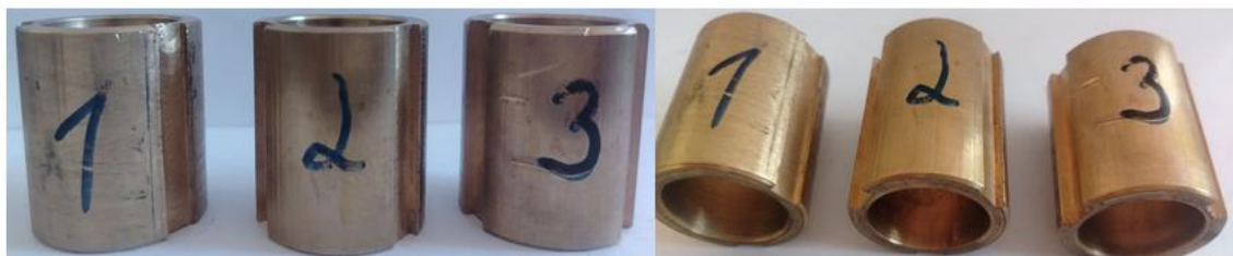
Figure 2. Inner bushing of the working body support structure for a vertical shaft machine.
