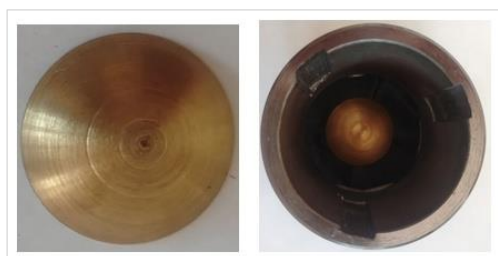
Figure 4. Spherical surface under the base plate of the working body support structure for a vertical shaft machine.
