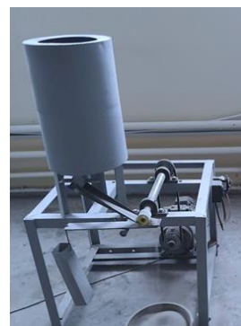
Figure 3. Device for testing materials for abrasive wear.
