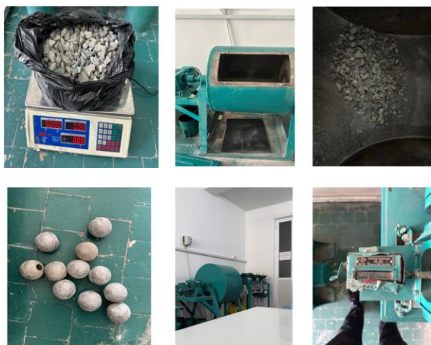
Figure 3. Determination of abrasion resistance (wear coefficient) of rock samples.
