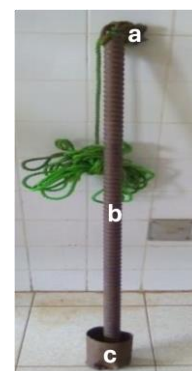
Figure 2. Fecal sludge sampling device (a: string; b: metal bar; c: graduated string).
