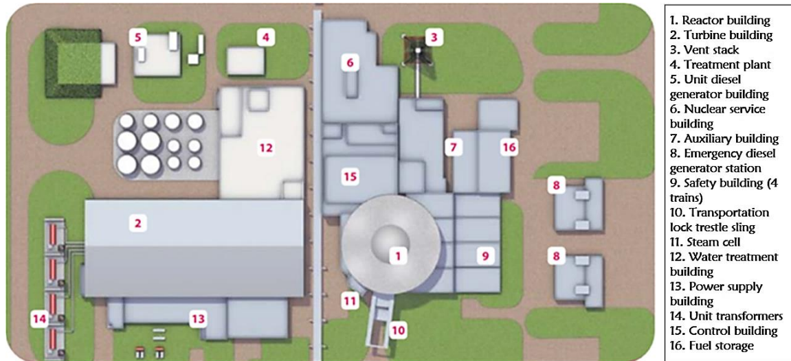
Figure 3. Schematic layout of a typical VVER plant at Rooppur Nuclear Power Plant [11].
