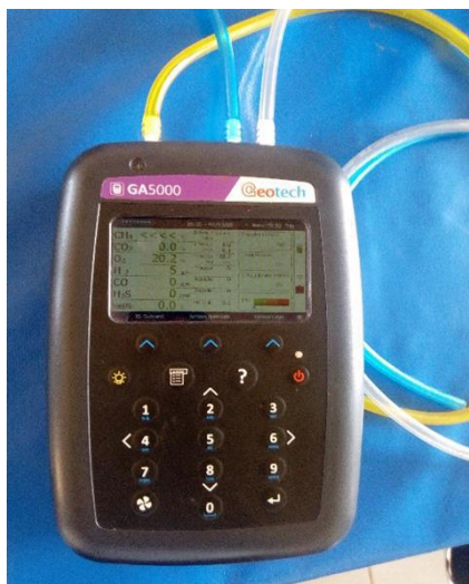
Figure 3. GA 5000q Portable Analyzer.
