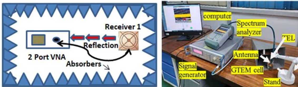
Figure 7. Measurement setup (a). Reflection coefficient S_{11} (b) E- Field Measurement in TEL.
