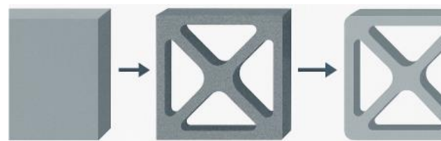
Figure 9. Illustration of topology optimization process: (a) Initial design domain, (b) material distribution after optimization, (c) manufacturable geometry.
