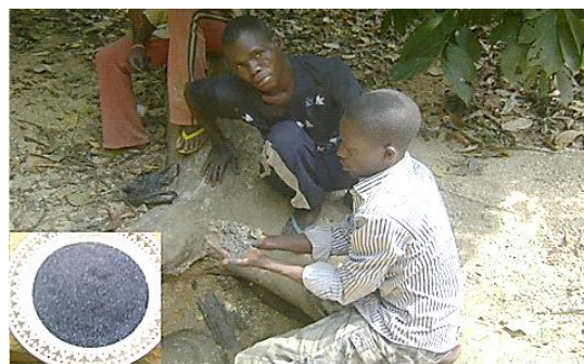
Figure 21. Stream sediments containing ilmenite at River Akpo (insert Panned ilmenite at River Akpo).
