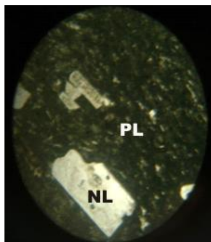
Figure 19. Basalt under cross polar.
